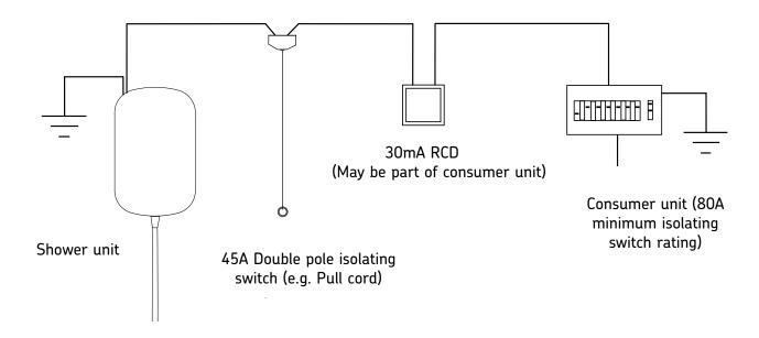
For adequate circuit protection DO NOT use a rewire-able fuse. Instead use a suitably rated miniature circuit breaker or cartridge fuse.
