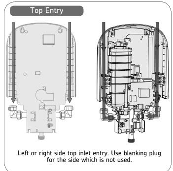
Note - Some water from the factory testing may escape when the blanking plugs are removed.
