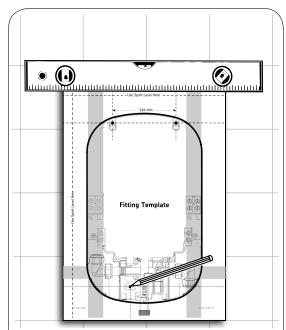
Ensure the template is level and temporarily hold in position with tape. Mark the 3 fixing points on the wall
