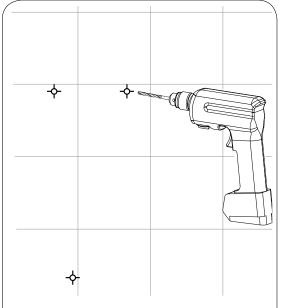
Remove the fitting template from the wall and drill the marked fixing points. Before drilling, ensure there are no cables or water supplies running within the wall
