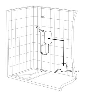
To connect the pump using wired connectivity, please follow the diagram shown. If you wish to connect the pump to the shower wirelessly, an optional wireless pump module is required. Please enquire using stock code: 29014 as a reference.
