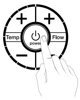
Confirm the operation of the Temperature and Flow increase and decrease buttons, whilst ensuring all lights are functioning
